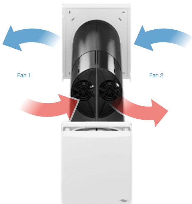
The iV Twin+ combines two decentralised fans in one. With the double guiding vanes, double Xenion® fan and double ceramic heat accumulator – all consistently separated vertically – it provides optimum moisture protection.
