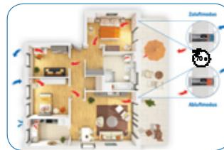
The ventilation unit operates on the principle of heat recovery by changing the direction of the fan. The integrated thermal accumulator charges itself with heat energy from the room's air as it flows to the exterior (extract air). After 70 seconds, each Xenion reversible fan changes direction. When the reversible fan changes direction, it releases the stored heat energy into the incoming outside air (supply air).
