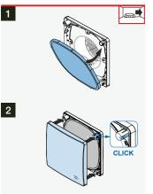
Insert the dust filter into the base plate.
